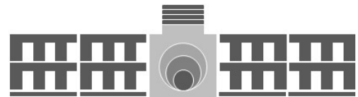
Alignment of the open backs of the RAUSIKKO Box LT basic elements to the C3 Type X
