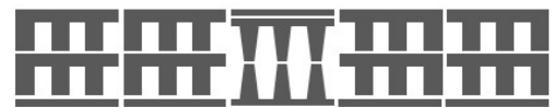
Alignment of the open backs of the RAUSIKKO Box LT basic elements to the RAUSIKKO Box SX
