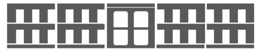
Alignment of the open backs of the RAUSIKKO Box LT basic elements to the RAUSIKKO Box S/SC
